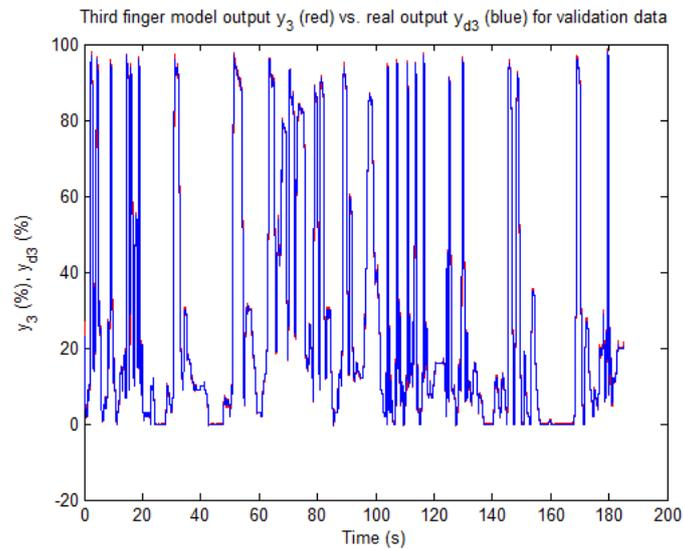
**Fig. 9.** Finger angle  $y_3$  versus time of TSK fuzzy model 7 (red) and real-world system (blue) on validation data set.
