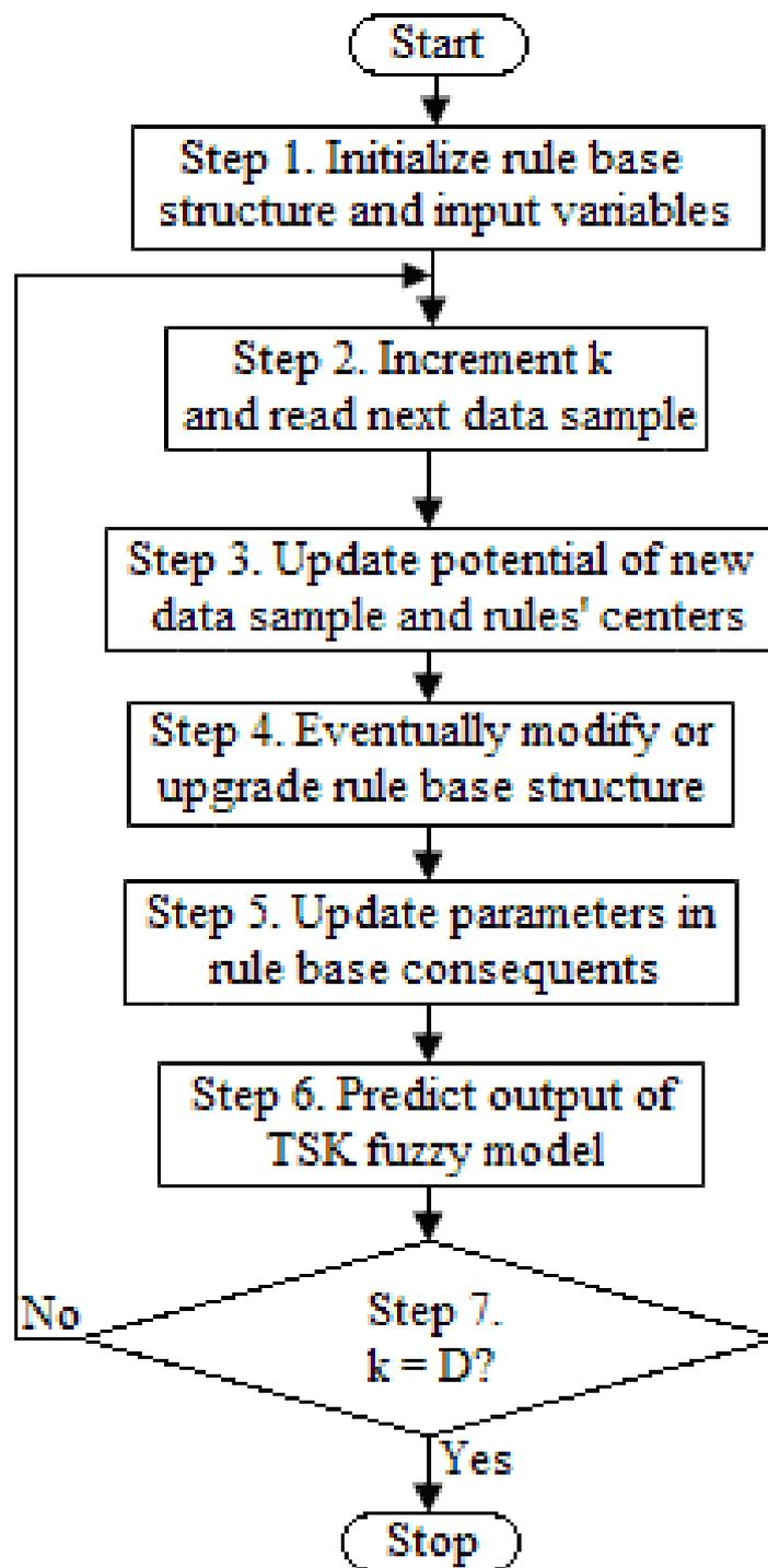
Fig. 1. Flowchart of incremental online identification algorithm [30].
