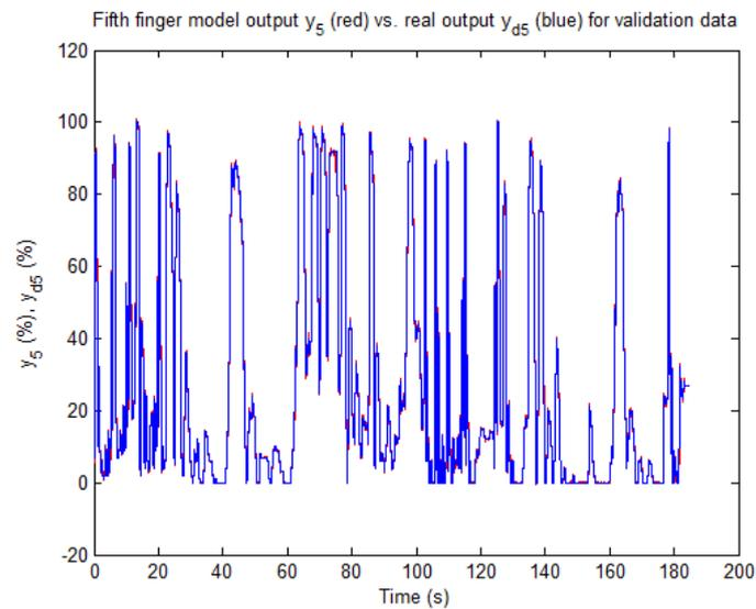
**Fig. 10.** Finger angle  $y_5$  versus time of TSK fuzzy model 7 (red) and real-world system (blue) on validation data set.
