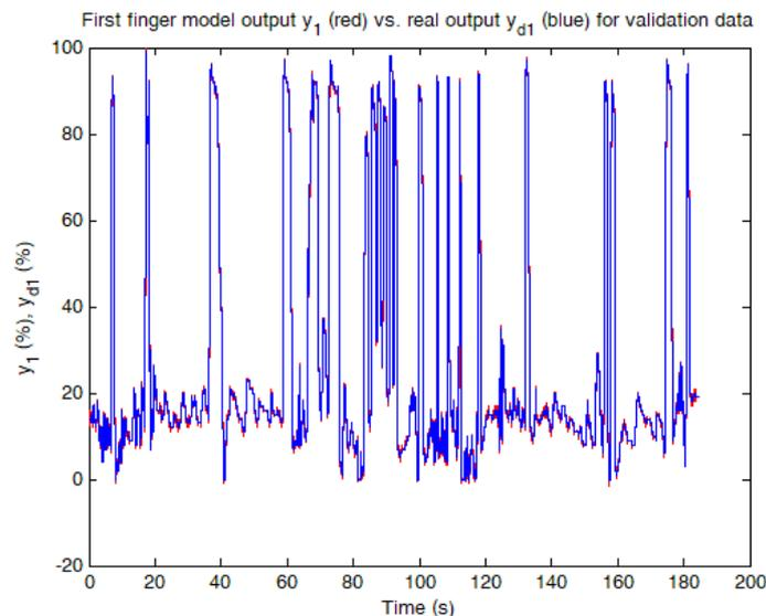
**Fig. 8.** Finger angle  $y_1$  versus time of TSK fuzzy model 7 (red) and real-world system (blue) on validation data set.
