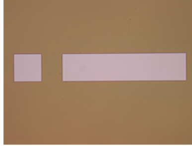
Fig. 4. The configuration of Source and the Drain as lateral electrode with larger surface.
