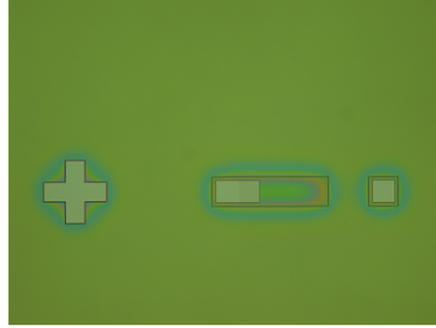
Fig. 5. The final p-NOI structure at optical microscope.
