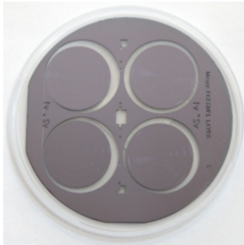
Fig. 5. Image of the Fresnel lenses separated from the wafer by a DRIE Bosch etching
