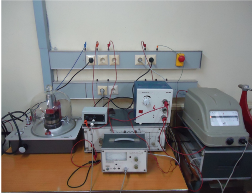
Fig. 2. Measuring circuit of the volume resistivity.
