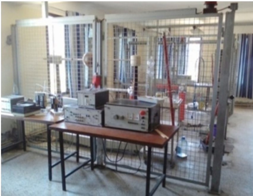
Fig. 3. Circuit of breakdown voltage tests.
