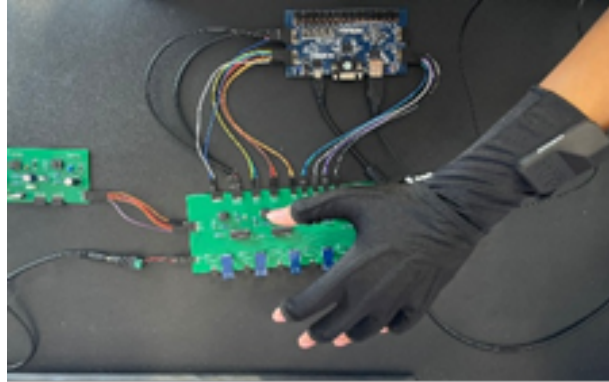
Fig. 5. The glove's interface for acquiring the fingers' movements parameters.
