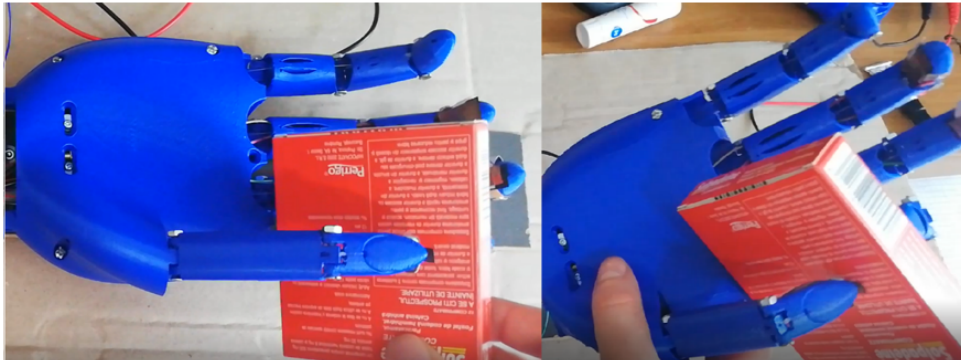
Fig. 9. Testing the algorithm of grasping an object with two fingers.
