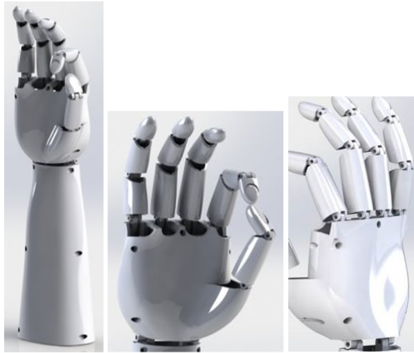
Fig. 1. The 3D-printed mechanical structure with anthropomorphic appearance.
