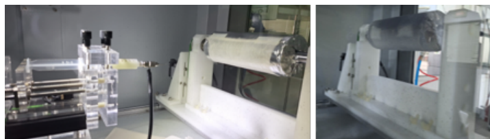
Fig. 2. a) The electrospinning system Nano Fiberlabs E05; b) The bandage after the process is done.
